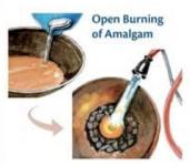
Mercury and gold form an amalgam, which is heated to evaporate the mercury. The mercury vapor released is highly toxic.
