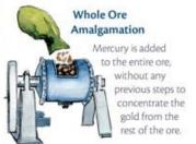
Mercury use is high and inefficient, often resulting in large amounts of mercury being lost to the mine tailings.
